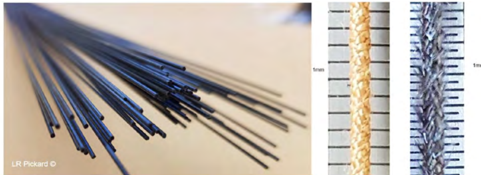
Figure 4. Micro overbraiding of pultruded rods. Left: carbon-fibre epoxy rods of 0.8 mm diameter. Centre: rod with 273 dtex PBO overbraid. Right: Rod with 1k T300 fuzzy carbon overbraid [4].
